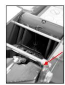
2. Rotate the release handle to the raised position.
