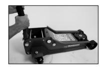
3. With the help of an assistant stand the jack on its end on the edge of a bench.
