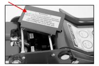
Insert the lower handle half into the handle socket and wind anticlockwise till the universal joint comes out of the hydraulic block. If the universal is broken use pliers or multigrips to wind the remaining section from the hydraulic block.
