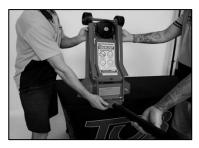
4. While holding the jack by the front axle slowly pump the lift arm out to full height.
